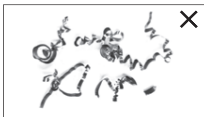
Apple-peel-like chips (Without curling)
